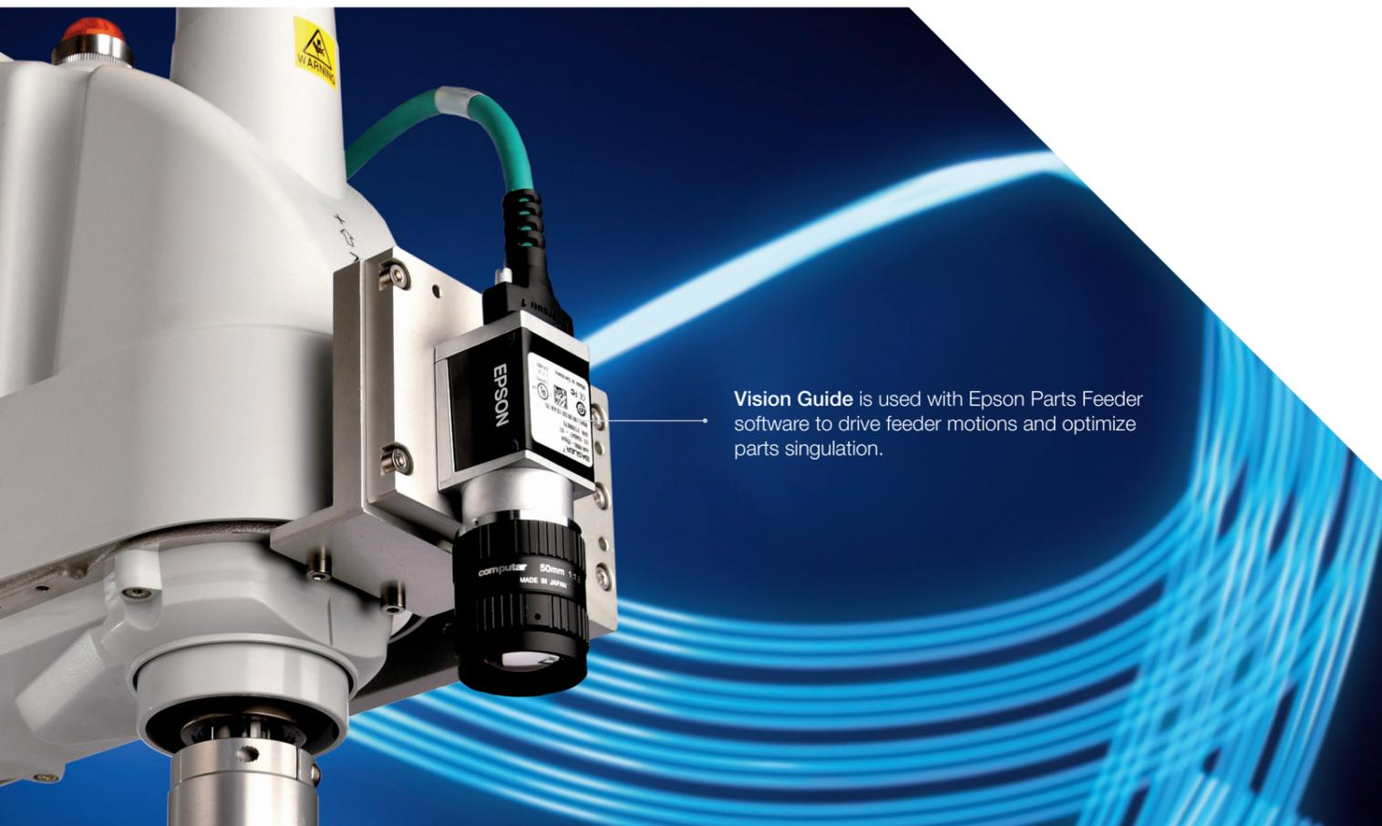
Vision Guide is used with Epson Parts Feeder software to drive feeder motions and optimize parts singulation.
