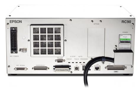
The Epson RC90 is the most compact and lightweight controller of its performance class on the market. The small smart one of extremely good value was mainly designed for slave network operation. Basically serial interface RS-232C, 24/16 standard I/O and Ethernet port are already installed. The expansion cards for communication with external devices and for integration into fieldbus networks can flexibly expand your system according to your requirements at a low cost.
