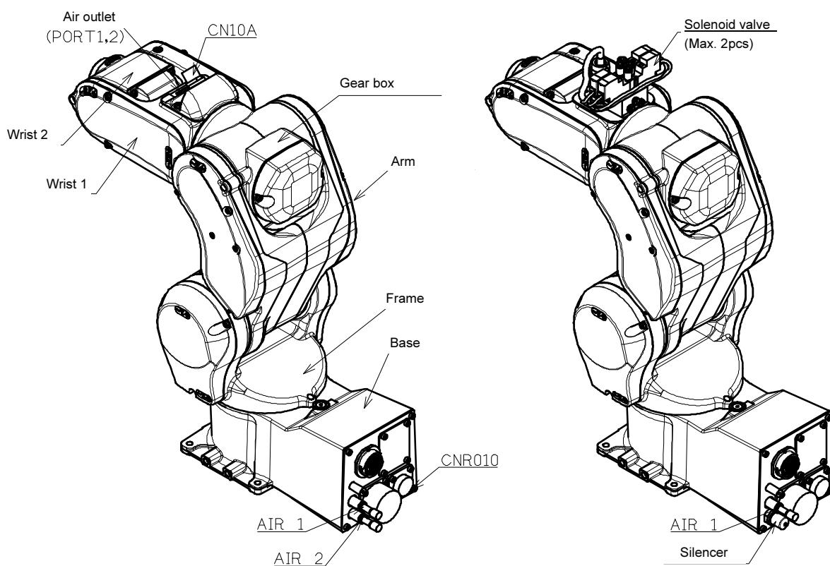
**Detailed diagram of the application connectors (standard)**
