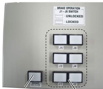
Power lamp Brake release switches
