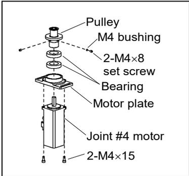
(2) Place the Joint #4 motor unit in the arm so that the motor cable faces toward the left from the end of Arm #2.
