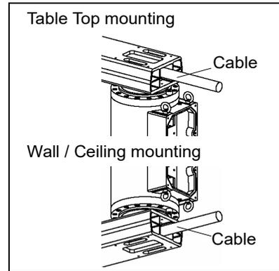
(20) Disconnect the Arm #2 side cables from the lower part of Arm #1.
