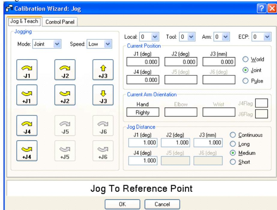
\* Position Joint #2 only and move Joint #3 to around 0 pulse.
