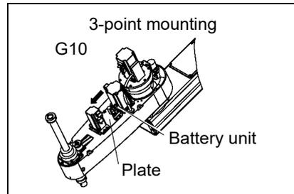
When you use the plate of 4-point mounting, you do not have to mount the plate.
