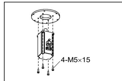
Joint #2 motor Installation
