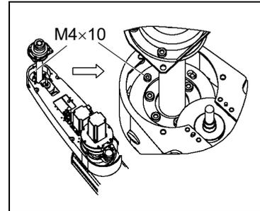
(3) Remove the reduction gear unit.
