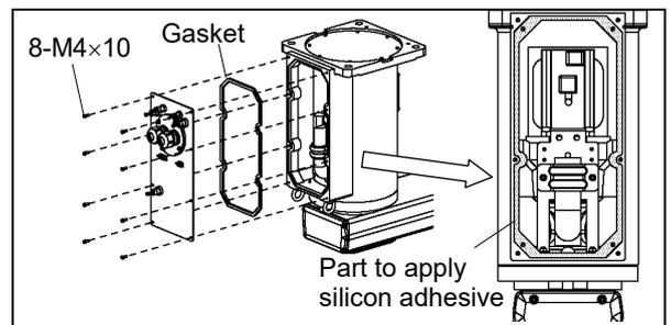
A gasket is installed to G10/G20-\*\*\*D\*, P\* (Protected-model).
