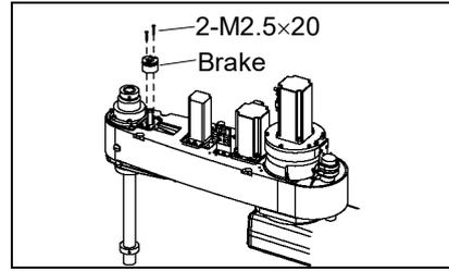
(2) Secure the brake hub with the two set screws.
