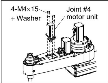
(4) Loosely secure the Joint #4 motor unit to Arm #2.
