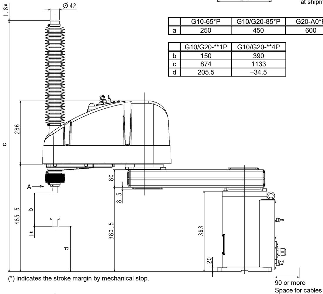
(\*) indicates the stroke margin by mechanical stop.
