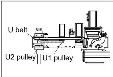
(5) Apply the proper tension to the U belt, and then secure the Joint #4 motor unit.
