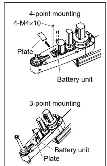
When you use the plate of 3-point mounting, loosen the plate mounting bolts.
