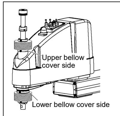
Attach the mounting part of the bellows until the end touches the cylindrical part of the cover.
