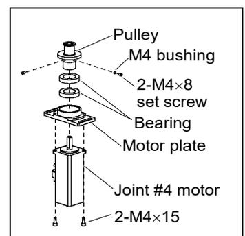
Joint #4 motor Installation: G10 (1) Mount the U1 pulley and the motor plate to the new Joint #4 motor.
