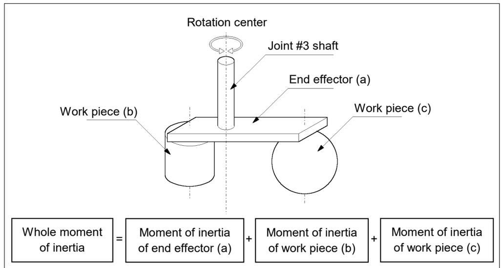
The methods for calculating the moment of inertia for (a), (b), and (c) are shown below. Calculate the total moment of inertia using the basic formulas.
