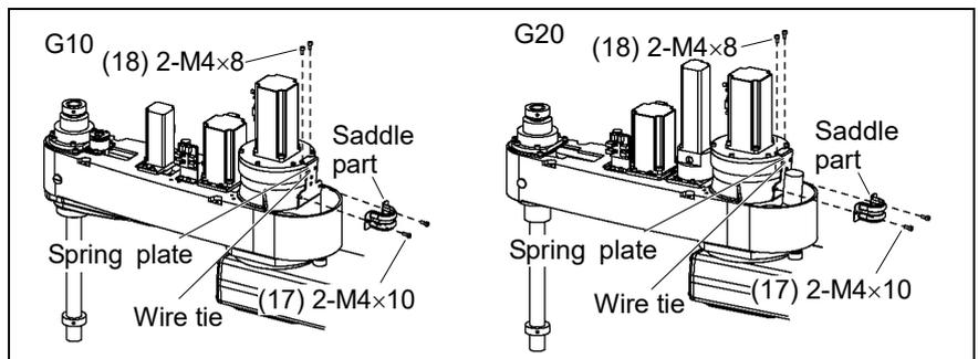
(17) Cut off the two wire tie binding cables.
