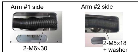
(23) Disconnect the cables to the base side.
