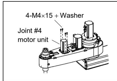
(4) When you use the plate of 3-point mounting, mount the plate with pressing it to the Joint #4 motor.
