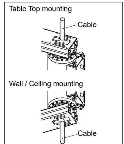
(19) Disconnect the cables that were disconnected from Arm #1 in step (18) to the side of Arm #1.
