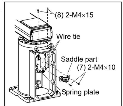
When using Wall mounting type
