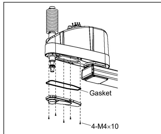
A gasket is installed to G10/G20-\*\*\*C\* (Cleanroom-model) and G10/G20-\*\*\*D\*/P\* (Protected-model).
