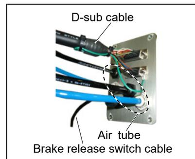
Be sure to observe the connection for connecting the disconnected parts after replacement.
