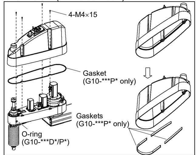
Gaskets are installed to G10-\*\*\*P\*.
