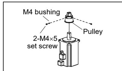
Joint #3 motor Installation
