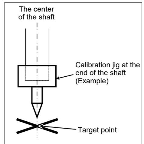
After removing the end effector and performing the calibration, install the end effector and move the Manipulator to the teaching point to verify whether there is a positional gap. If there is a positional gap, fine-tune the installation position of the end effector and teach the point again.
