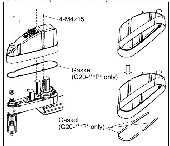
Gaskets are installed to G20-\*\*\*P\*.
