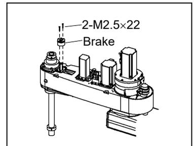
Joint #4 brake (1) Mount the brake.
