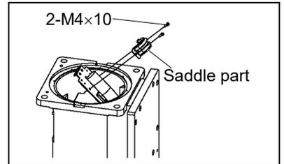
(6)-3 Loosely band the cables with a wire tie. Be sure to keep the wire tie loose enough so that the cables move.
