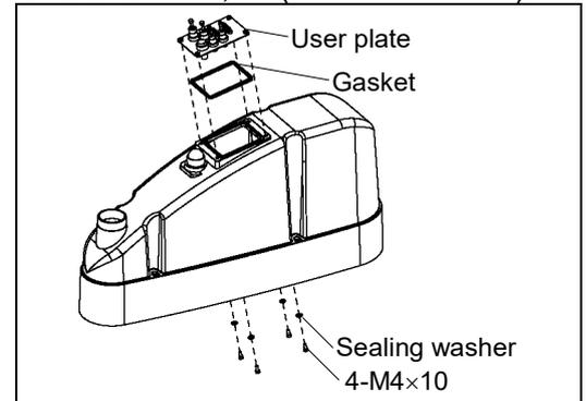
A gasket and sealing washers are installed to G10/G20-\*\*\*D\*, P\* (Protected-model).
