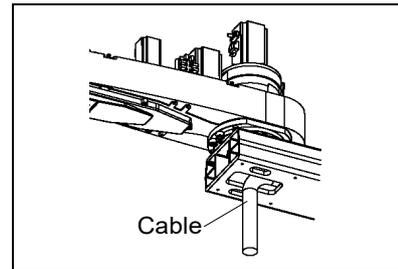
(21) Disconnect the cables that were disconnected to the lower part of Arm #1 in step (20) to the side of Arm #1.
