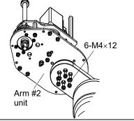
(6) Tighten the screw secured loosely in the step (4).
