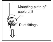
Cable unit Installation (1) Pass the cables through the user plate and secure the duct fittings.
