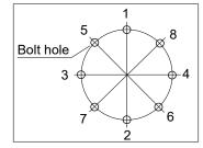
Do not fasten all bolts securely at one time. Divide the number of times that the bolts are fastened into two or three and fasten the bolts securely with a hexagonal wrench. Then, use a torque wrench so that the bolts are fastened with tightening torques shown in the table above.
