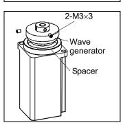
Joint #2 motor(1)Mount the motor spacer and wave generator on theInstallationJoint #2 motor.
