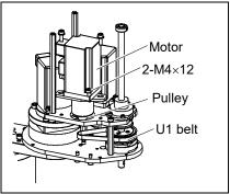
(9) Remove the motor from the Joint #4 motor housing.
