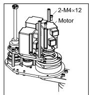
(6) Remove the wave generator and motor spacer.
