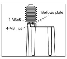
(11) Pull out the upper bellows from the bellows plate.
