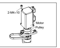
Joint #3 motor(1)Mount the brake hub and pulley to the new motorInstallationshaft.
