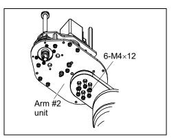
(5) Remove the screw secured loosely in the step(3) and also remove the Joint #2 motor flange, reduction gear, and Joint #2 spacer.
