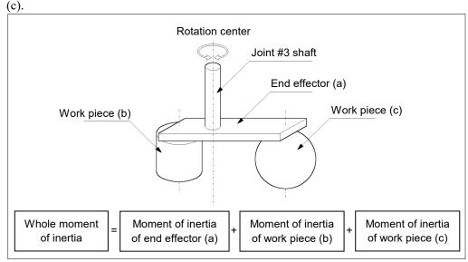
The methods for calculating the moment of inertia for (a), (b), and (c) are shown below. Calculate the total moment of inertia using the basic formulas.
