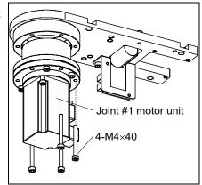
(6) Loosen the screw fixing the motor flange and reduction gear and remove the motor unit.
