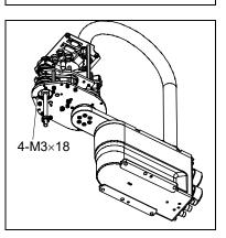
(11) Pull out the ball screw spline unit from Arm #2.
