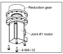
(7) Remove the wave generator from the Joint #1motor.
