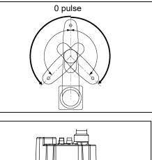
0 pulse position of Joint #3: upper limit position in motion range
