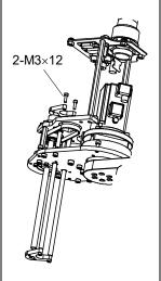
Loosely secure the upper side of support shaft to the upper support guide. After moving the shaft up and down several times, secure the set screw on the upper side of shaft, and then secure the set screw of the lower support guide.
