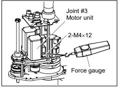
(5) Perform the calibration of Joint #3.For details, refer to *Maintenance: 13. Calibration*.
