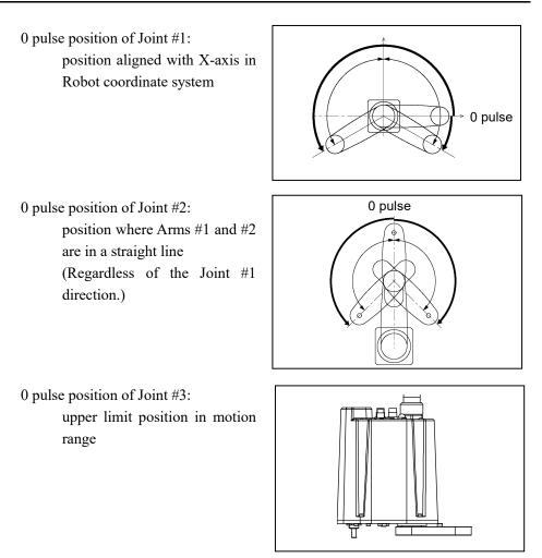
The height of Joint #3 depends on manipulator model.
