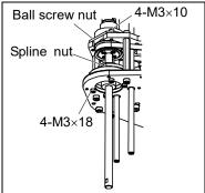
(6) Pull out the U belt and ball screw spline unit from Arm #2.
