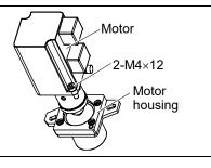
(10) Remove the pulley from the Joint #4 motor.
