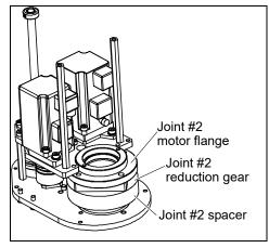
Joint #2 reduction gear unit Installation
