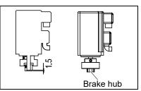
After the brake hub is mounted, press the pulley lightly to the brake hub and secure.
