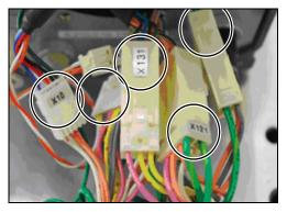
M/C Cable Installation (1) Connect new M/C cable connectors to those of the Cable Unit.
