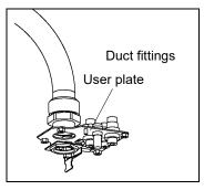
(11) Remove the connector plate.
