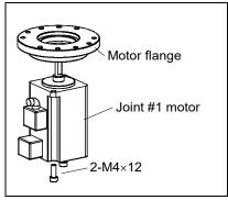
(2) Mount the waveform generator on the Joint #1 motor.
