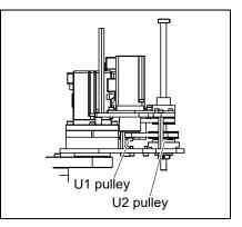
(6) Apply the proper tension to the U1 belt, and then secure the Joint #4 motor unit.
