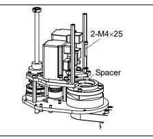
(3) Loosen the screw fixing the Joint #2 reduction gear unit and loosely secure.
