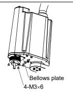
Bellows Installation (4-axis spec)
