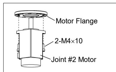
Joint #2 Motor Installation
