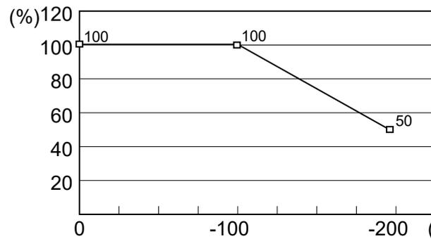
\* Figures on the graph (%) are the proportion to the acceleration/deceleration speed at the shaft upper limit position.
