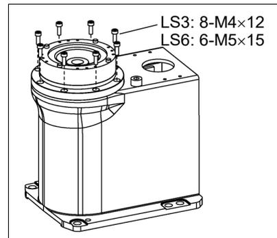
(6) LS3: Loosen the motor mounting screws on the Joint #1 motor flange and remove the motor unit
