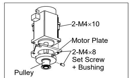
Joint #4 motor Installation
