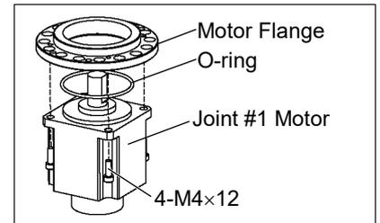
Joint #1 motor Installation
