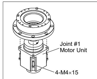
LS6: Loosen the motor flange mounting screws on the Joint #1 motor flange and remove the motor unit
