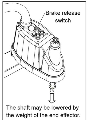
This button switch is a momentary-type; the brake is released only while the button switch is being pressed.
