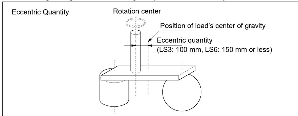
**Eccentric quantity of load on the shaft**
