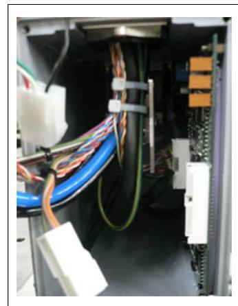
(5) Disconnect the connectors X10 and X20 from the resolver board.
