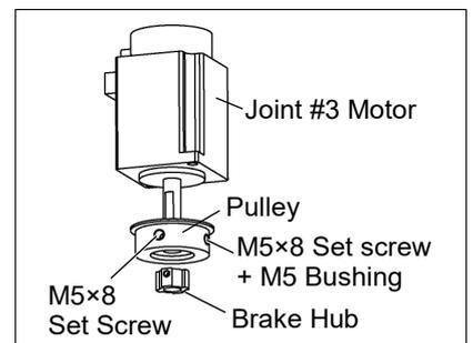
Joint #3 motor Installation
