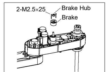
For LS6 series (1) Mount the brake to the Joint #4 intermediate shaft unit.
