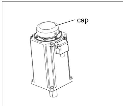
(3) Loosely secure the Joint #3 motor unit to Arm #2.
