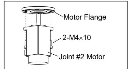
(2) Mount the waveform generator on the Joint #2 motor.
