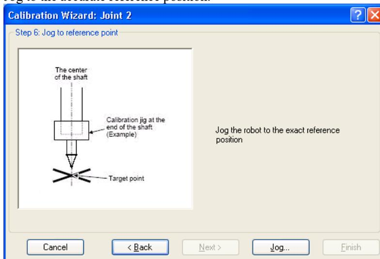
Jog to the accurate reference position and adjust the position. Click the <OK> button.
